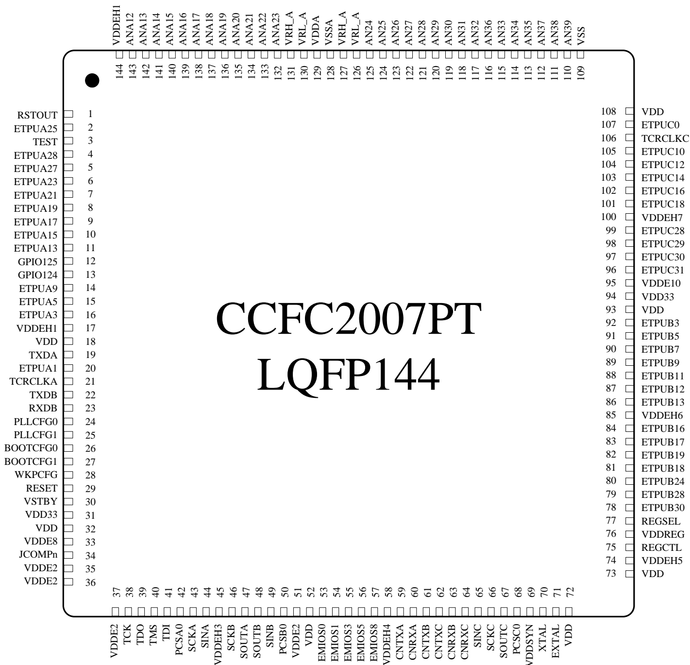
Figure 5. CCFC2007PT 144-pin LQFP
